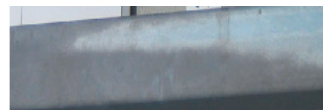
Differences in colour may exist, but do not influence on the quality of the corrosion protection. The reason for the differences is that the reaction between steel and iron varies depending on type of steel and cooling speed after galvanizing.
